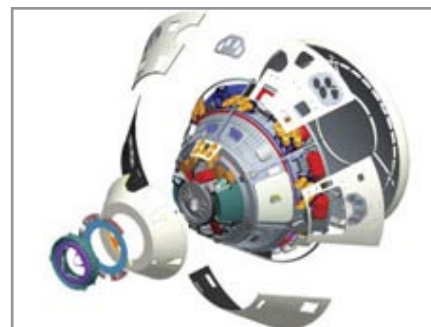
Figure 3: Exploded view of Orion. Image Credit: Lockheed Martin Corp
